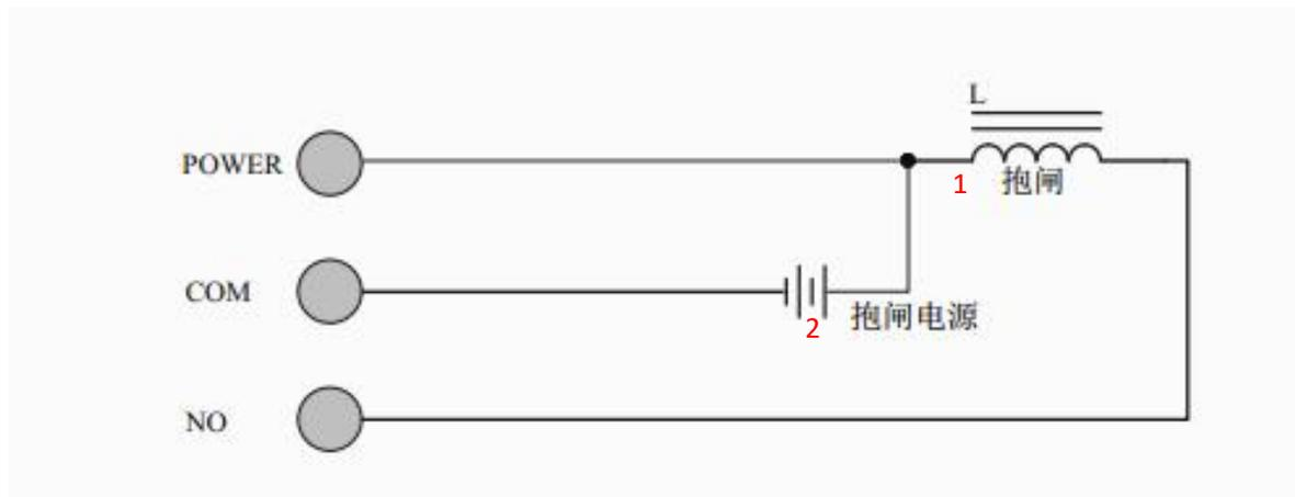
Schematic Diagram of MINI Drive Brake Wiring
